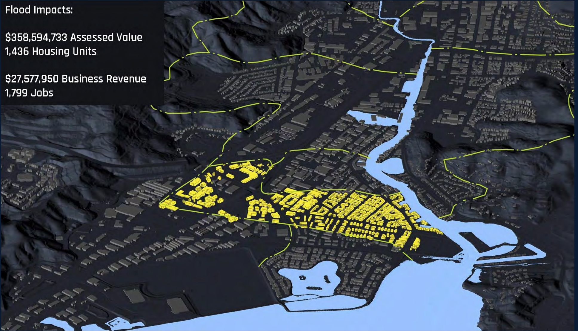
Flood Impacts with a Single Pump Failure
