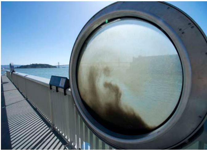
Bay Window – One of a series of discs holding Bay water and sediment collected from different parts of the Bay, may be spun to see sediment distribution/turbidity.
