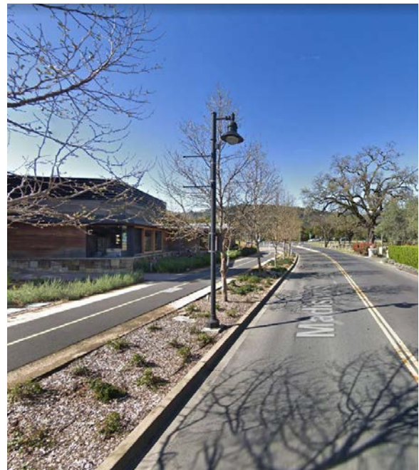
Madison Street in Yountville, CA incorporates a separated cycle-track, planted buffer with canopy trees, lighting, a planted buffer, and narrow travel lanes. This streetscape contributes to a comfortable pedestrian and cycling experience.
