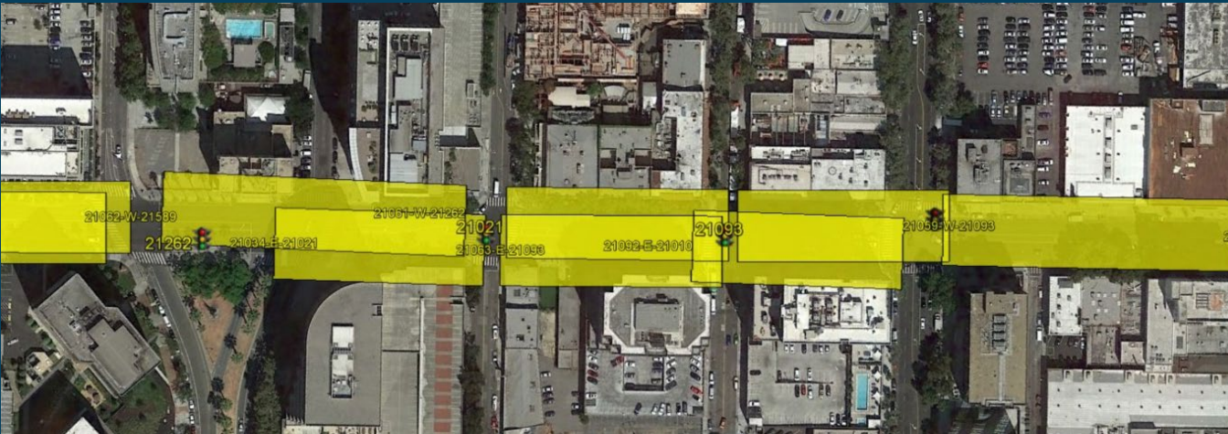
Bounding boxes for hardware-based TSP system on Santa Clara Street
